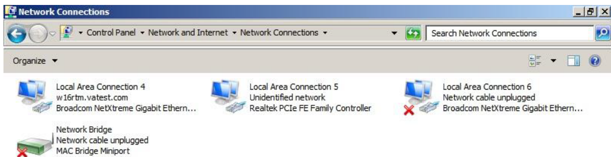
Image 1.8: Example of a network configuration that needs to be corrected
